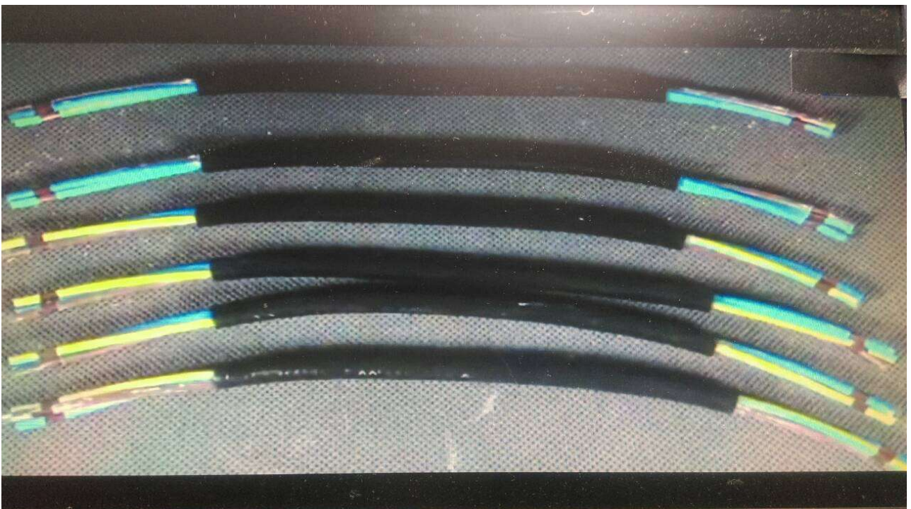
Cutting and Stripping samples :
